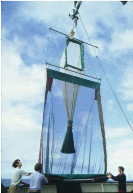
Figure 2. An opening/closing Rectangular Midwater Trawl system (RMT1+8). The lower net has an 8m 2 mouth area and mesh of 4.5mm, the upper one a mouth area of 1m 2 and a mesh of 0.33mm. This combination allows a wider size range to be sampled than would be possible with a single net. The nets open and close simultaneously on receipt of an appropriate acoustic signal from the ship. (Photo: Southampton Oceanography Centre)
